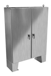
Hammond enclosure, NEMA 3R/4X/12/13, 72 x 60 x 18in (HxWxD), floor mount, 316 stainless steel, #4 brush finish, 2-door, 3-point 316 stainless steel padlocking handle.
