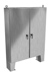
Hammond enclosure, NEMA 3R/4X/12/13, 72 x 60 x 12in (HxWxD), floor mount, 316 stainless steel, #4 brush finish, 2-door, 3-point 316 stainless steel padlocking handle.
