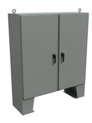
Hammond enclosure, NEMA 3R/4/12/13, 60 x 60 x 18in (HxWxD), floor mount, carbon steel, ANSI 61 gray, powder coat finish, 2-door, 3-point padlocking handle.
