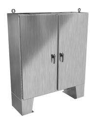
Hammond enclosure, NEMA 3R/4X/12/13, 60 x 60 x 18in (HxWxD), floor mount, 304 stainless steel, #4 brush finish, 2-door, 3-point 316 stainless steel padlocking handle.
