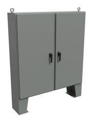
Hammond enclosure, NEMA 3R/4/12/13, 60 x 60 x 12in (HxWxD), floor mount, carbon steel, ANSI 61 gray, powder coat finish, 2-door, 3-point padlocking handle.
