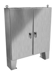
Hammond enclosure, NEMA 3R/4X/12/13, 60 x 60 x 12in (HxWxD), floor mount, 304 stainless steel, #4 brush finish, 2-door, 3-point 316 stainless steel padlocking handle.
