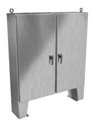
Hammond enclosure, NEMA 3R/4X/12/13, 60 x 60 x 12in (HxWxD), floor mount, 316 stainless steel, #4 brush finish, 2-door, 3-point 316 stainless steel padlocking handle.
