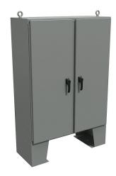
Hammond enclosure, NEMA 3R/4/12/13, 60 x 48 x 18in (HxWxD), floor mount, carbon steel, ANSI 61 gray, powder coat finish, 2-door, 3-point padlocking handle.
