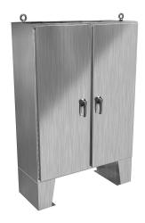
Hammond enclosure, NEMA 3R/4X/12/13, 60 x 48 x 18in (HxWxD), floor mount, 304 stainless steel, #4 brush finish, 2-door, 3-point 316 stainless steel padlocking handle.
