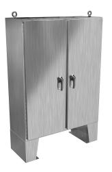
Hammond enclosure, NEMA 3R/4X/12/13, 60 x 48 x 18in (HxWxD), floor mount, 316 stainless steel, #4 brush finish, 2-door, 3-point 316 stainless steel padlocking handle.
