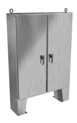
Hammond enclosure, NEMA 3R/4X/12/13, 60 x 48 x 12in (HxWxD), floor mount, 316 stainless steel, #4 brush finish, 2-door, 3-point 316 stainless steel padlocking handle.
