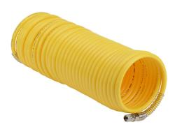
NITRA pneumatic coiled hose, nylon 12, yellow, 3/8in inside diameter, 0.47in outside diameter, (2) 3/8in male NPT nickel-plated brass swivel fittings, 42ft working length.
