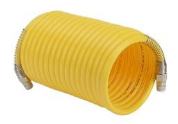
NITRA pneumatic coiled hose, nylon 12, yellow, 3/8in inside diameter, 0.47in outside diameter, (2) 3/8in male NPT nickel-plated brass swivel fittings, 20ft working length.
