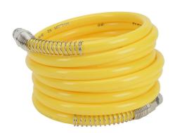
NITRA pneumatic coiled hose, nylon 12, yellow, 3/8in inside diameter, 0.47in outside diameter, (2) 3/8in male NPT nickel-plated brass swivel fittings, 10ft working length.
