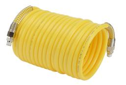
NITRA pneumatic coiled hose, nylon 12, yellow, 3/8in inside diameter, 0.47in outside diameter, (2) 1/4in male NPT nickel-plated brass swivel fittings, 20ft working length.
