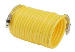
NITRA pneumatic coiled hose, nylon 12, yellow, 3/8in inside diameter, .47in outside diameter, (2) 1/4in male NPT nickel-plated brass swivel fittings, 20ft working length.
