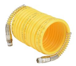
NITRA pneumatic coiled hose, nylon 12, yellow, 1/4in inside diameter, 0.3125in outside diameter, (2) 1/4in male NPT nickel-plated brass swivel fittings, 10ft working length.
