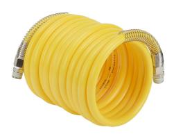
NITRA pneumatic coiled hose, nylon 12, yellow, 1/2in inside diameter, 0.625in outside diameter, (2) 1/2in male NPT nickel-plated brass swivel fittings, 20ft working length.
