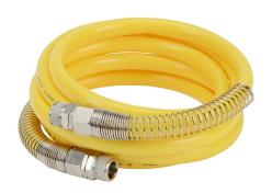
NITRA pneumatic coiled hose, nylon 12, yellow, 1/2in inside diameter, 0.625in outside diameter, (2) 1/2in male NPT nickel-plated brass swivel fittings, 10ft working length.
