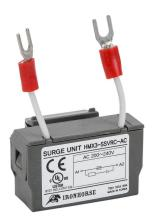
IronHorse surge suppressor, varistor-resistor-capacitor, 200-240 VAC. For use with HMC-9 to HMC-150 contactors.
