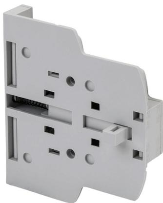
IronHorse field installable auxiliary contact, left or right side mount, (1) N.O./ (1) N.C. contact(s), 6A @ 120 VAC/1.1A @ 120 VDC, screw terminal. For use with HMC-185 to HMC-400 contactors.
