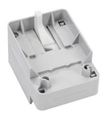
IronHorse mechanical interlock, side mount. For use with HMC-185 to HMC-400 contactors. Allows for mechanical connection of two contactors to prevent both from being pulled in at the same time.
