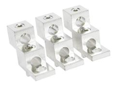
IronHorse box type wiring lug, line or load mount, 2 openings, #3 AWG-4/0 MCM wire(s). Package of 3. For use with HMC-265 to HMC-400 contactors.
