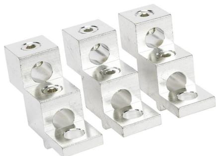
IronHorse box type wiring lug, line or load mount, 2 openings, #3 AWG-4/0 MCM wire(s). Package of 3. For use with HMC-265 to HMC-400 contactors.
