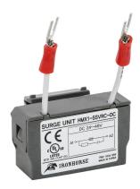
IronHorse surge suppressor, varistor-resistor-capacitor, 24-48 VDC. For use with HMC-9 to HMC-150 contactors.
