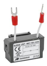
IronHorse surge suppressor, varistor, 24-48 VAC/VDC. For use with HMC-9 to HMC-150 contactors.
