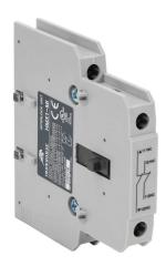
IronHorse mechanical interlock, side mount. For use with HMC-9 to HMC-150 contactors. Allows for mechanical connection of two contactors to prevent both from being pulled in at the same time.
