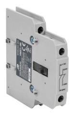
IronHorse mechanical interlock, side mount. For use with HMC-9 to HMC-150 contactors. Allows for mechanical connection of two contactors to prevent both from being pulled in at the same time.
