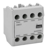
IronHorse field installable auxiliary contact, front mount, (4) N.O. contact(s), 6A @ 120 VAC/0.55A @ 120 VDC, screw terminal. For use with HMC-9 to HMC-150 contactors.
