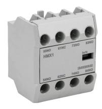
IronHorse field installable auxiliary contact, front mount, (3) N.O./ (1) N.C. contact(s), 6A @ 120 VAC/0.55A @ 120 VDC, screw terminal. For use with HMC-9 to HMC-150 contactors.
