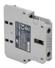
IronHorse field installable auxiliary contact, left or right side mount, (1) N.O./(1) N.C. contact(s), 6A @ 120 VAC/1.1A @ 120 VDC, screw terminal. For use with HMC-9 to HMC-150 contactors.
