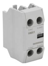
IronHorse field installable auxiliary contact, front mount, (1) N.O./ (1) N.C. contact(s), 6A @ 120 VAC/0.55A @ 120 VDC, screw terminal. For use with HMC-9 to HMC-150 contactors.
