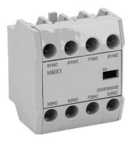
IronHorse field installable auxiliary contact, front mount, (4) N.C. contact(s), 6A @ 120 VAC/0.55A @ 120 VDC, screw terminal. For use with HMC-9 to HMC-150 contactors.
