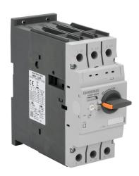
IronHorse manual motor protector, rotary, 50A, thermal overload, 34-50A adjustable, 650A instantaneous trip rating, 55mm frame.
