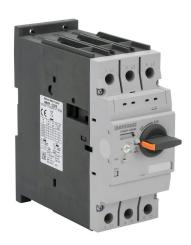
IronHorse manual motor protector, rotary, 40A, thermal overload, 28-40A adjustable, 520A instantaneous trip rating, 55mm frame.
