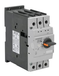
IronHorse manual motor protector, rotary, 32A, thermal overload, 22-32A adjustable, 416A instantaneous trip rating, 55mm frame.
