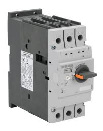
IronHorse manual motor protector, rotary, 26A, thermal overload, 18-26A adjustable, 338A instantaneous trip rating, 55mm frame.
