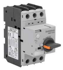
IronHorse manual motor protector, rotary, 8A, thermal overload, 5-8A adjustable, 104A instantaneous trip rating, 45mm frame.
