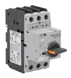
IronHorse manual motor protector, rotary, 4A, thermal overload, 2.5-4A adjustable, 52A instantaneous trip rating, 45mm frame.
