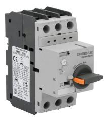
IronHorse manual motor protector, rotary, 40A, thermal overload, 28-40A adjustable, 520A instantaneous trip rating, 45mm frame.
