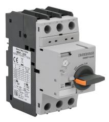
IronHorse manual motor protector, rotary, 26A, thermal overload, 18 -26A adjustable, 338A instantaneous trip rating, 45mm frame.
