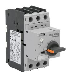
IronHorse manual motor protector, rotary, 22A, thermal overload, 14-22A adjustable, 286A instantaneous trip rating, 45mm frame.
