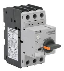
IronHorse manual motor protector, rotary, 2.5A, thermal overload, 1.6-2.5A adjustable, 32.5A instantaneous trip rating, 45mm frame.
