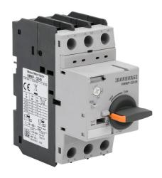
IronHorse manual motor protector, rotary, 1A, thermal overload, 0.63-1A adjustable, 13A instantaneous trip rating, 45mm frame.
