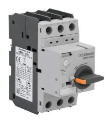
IronHorse manual motor protector, rotary, 17A, thermal overload, 11-17A adjustable, 221A instantaneous trip rating, 45mm frame.
