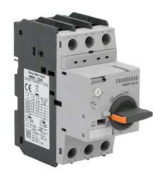
IronHorse manual motor protector, rotary, 10A, thermal overload, 6-10A adjustable, 130A instantaneous trip rating, 45mm frame.
