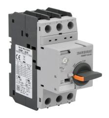
IronHorse manual motor protector, rotary, 0.4A, thermal overload, 0.25-0.4A adjustable, 5.2A instantaneous trip rating, 45mm frame.
