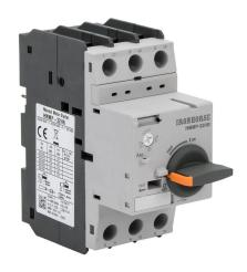
IronHorse manual motor protector, rotary, 0.25A, thermal overload, 0.16-0.25A adjustable, 3.3A instantaneous trip rating, 45mm frame.
