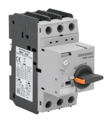
IronHorse manual motor protector, rotary, 0.16A, thermal overload, 0.1-0.16A adjustable, 2.1A instantaneous trip rating, 45mm frame.
