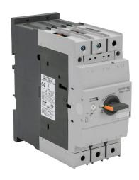
IronHorse manual motor protector, rotary, 90A, thermal overload, 70-90A adjustable, 1170A instantaneous trip rating, 70mm frame.
