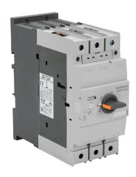
IronHorse manual motor protector, rotary, 75A, thermal overload, 55-75A adjustable, 975A instantaneous trip rating, 70mm frame.
