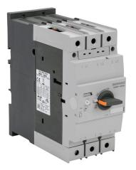
IronHorse manual motor protector, rotary, 100A, thermal overload, 80-100A adjustable, 1300A instantaneous trip rating, 70mm frame.
