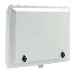
Stahlin SolarShield series HMI cover, NEMA 4/4X,  $17.33 \times 23.07 \times 2.59$ in, polycarbonate, Pantone 428 C glacier gray. For use with HMIs up to 14x20in (HxW).
